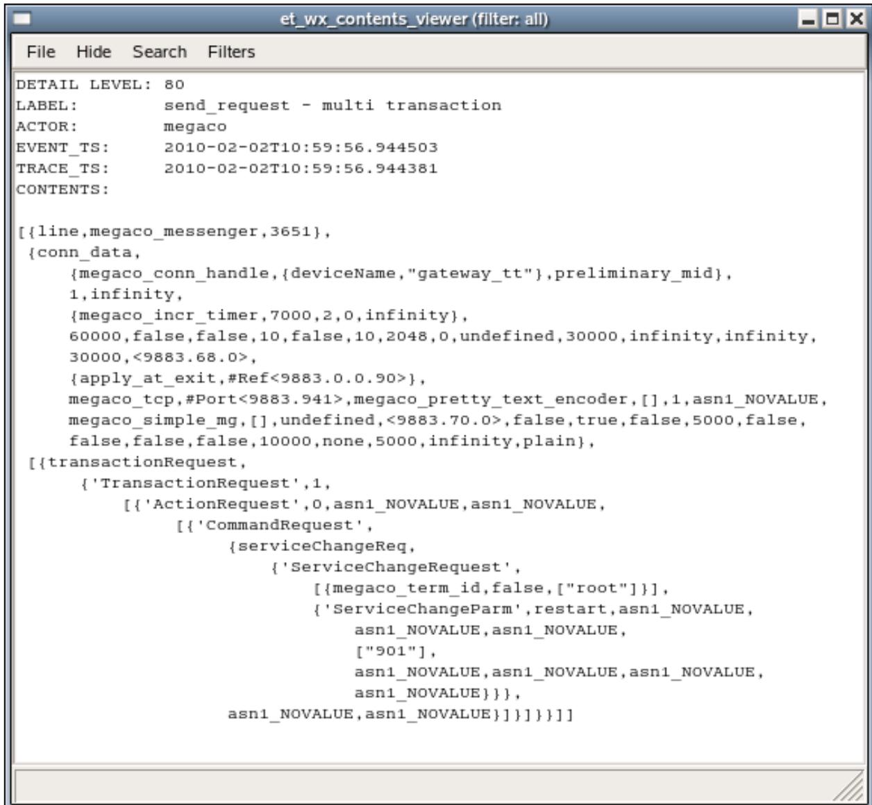
Figure 4.5: The internal form of a Megaco message
