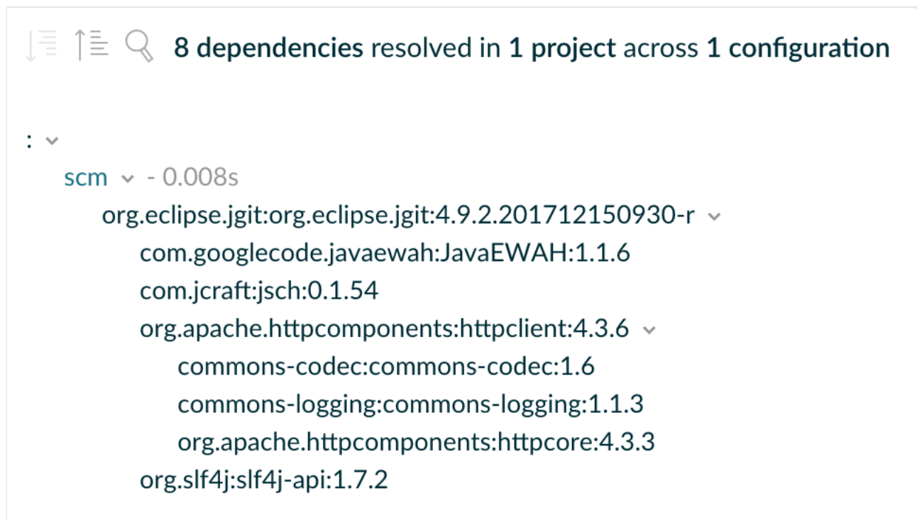
Figure 12. Dependency tree in a build scan
