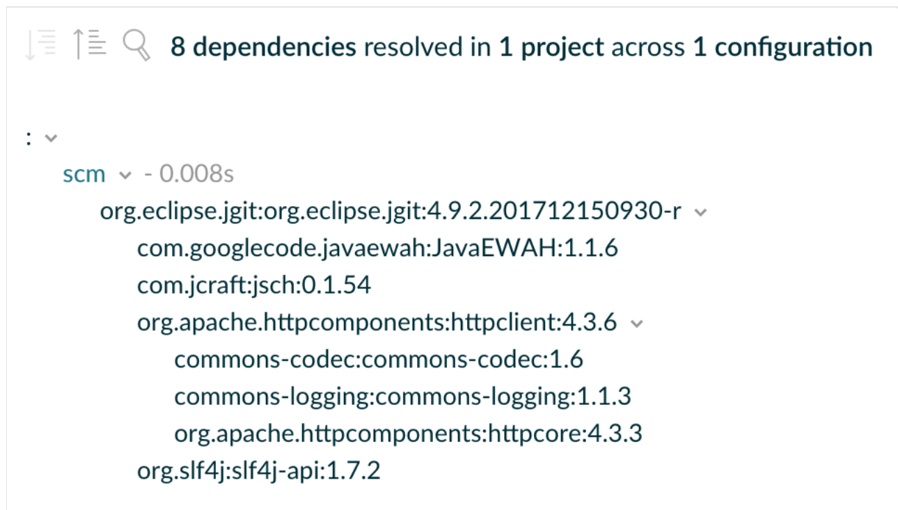
Figure 23. Dependency tree in a build scan
