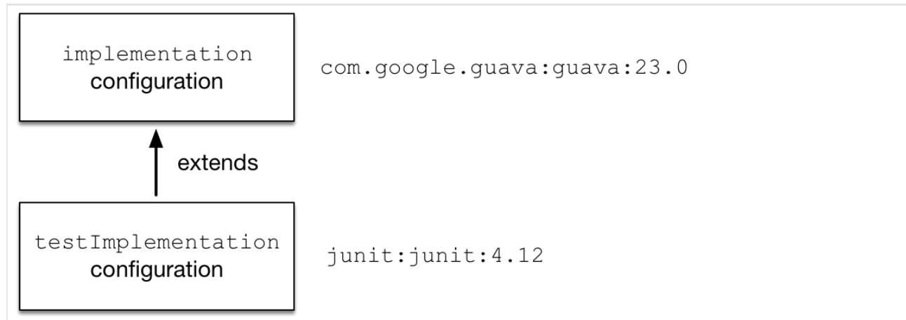
Figure 21. Configuration inheritance provided by the Java plugin
