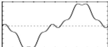
gi1 ftgen 1,0,2^10,9, 1,3,0, 3,1,0, 9,0.333,180 - approximation of a square wave
